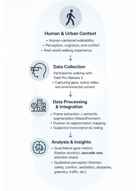
FIGURE 2 – Overview of the processing pipeline linking mobile eye-tracking, semantic segmentation, and segment-level walkability ratings.
